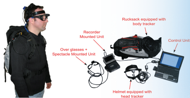
FIGURE 4 The Body Head Eye Movement System (BoHEM) consists of a motion-sensing helmet, rucksack, and spectacles. Body and eye movements in response to controlled stimuli are tracked and analyzed, allowing researchers to gain a comprehensive understanding of wearer's posture and direction of gaze.
