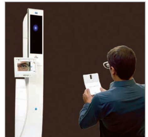
FIGURE 3 Determination of the leading dominant eye with the Visioffice® System Hand Held Measuring Device™. The determination is entirely automatic: no action on the part of the eyecare professional is required.
